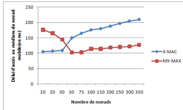
Figure 6. Average medium access delay of the mobile node
