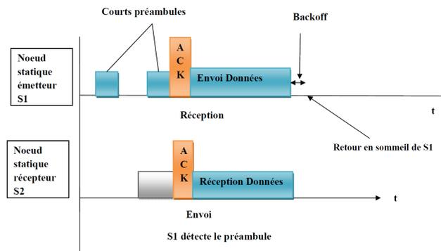
Figure 3. MX-MAC : operation where no mobile node access to the channel
