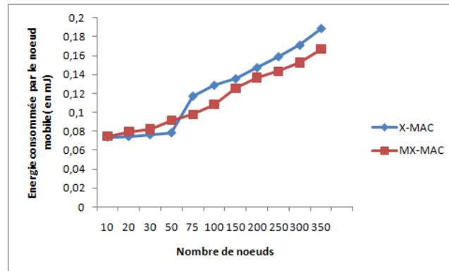
**Figure 4.** Average Energy consumed by the mobile node period of mobiles nodes relative to the static nodes in contrast with X-MAC protocol where static and mobile nodes are in competition for the channel access. Thus the small decrease in the rate of packet loss for MX-MAC compared to X-MAC is explained by the fact that a moving node has a high probability of data loss during communications due to synchronization errors that result.
